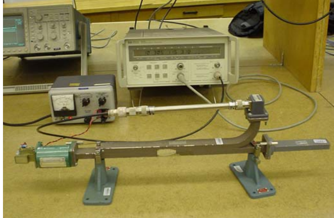
Fig. 3.9 The setup for the measurement of the frequency of the Gunn flange.
