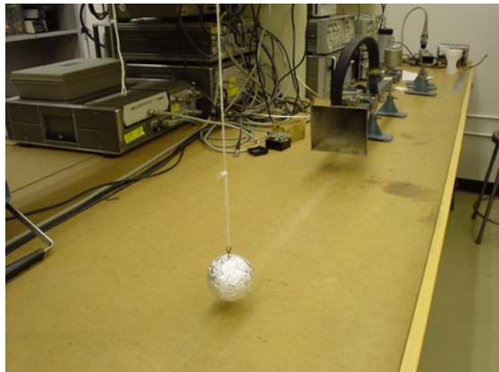
Figure 3.4 The foil-covered tennis ball swings in front of the horn antenna.
